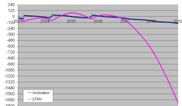
Figure 10. Foreseen inclination and LTAN evolution of Metop-A orbit; E option
