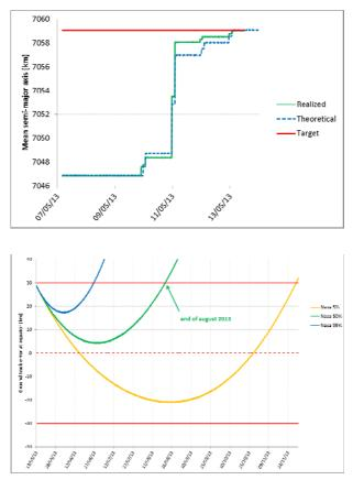
at the end, to limit the deviations while stopping the orbit drift on the targets. At the end of the transfer, the next OCM was expected around end of August 2013 (under typical 50-quantil solar activity conditions).
