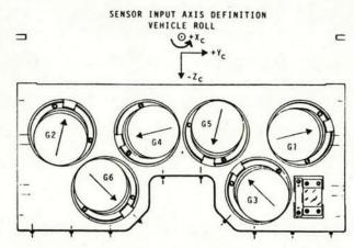
Figure 4. Gyro Input axes orientation
