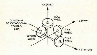
Figure 5. IUE wheel configuration
