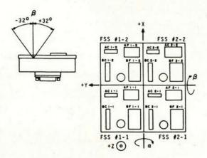
Figure 2. Fine Sun Sensor System
