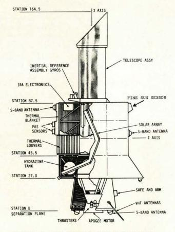
Figure 1. IUE Control axes & Features
