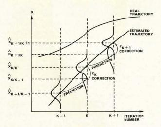
Figure 5. Orbit Determination Prediction - Correction
