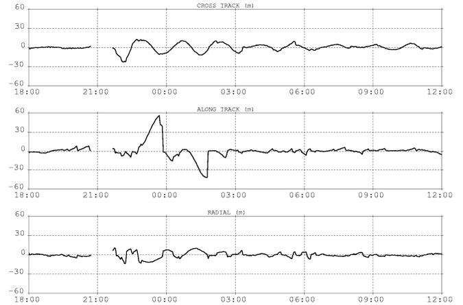
**Figure 3: DIODE-SPOT4 errors after a maneuver**
