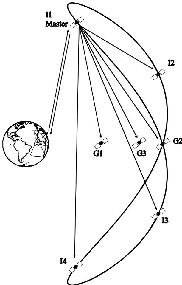
**Figure 4** GNSS-2 tracking with Master/Slave concept.
