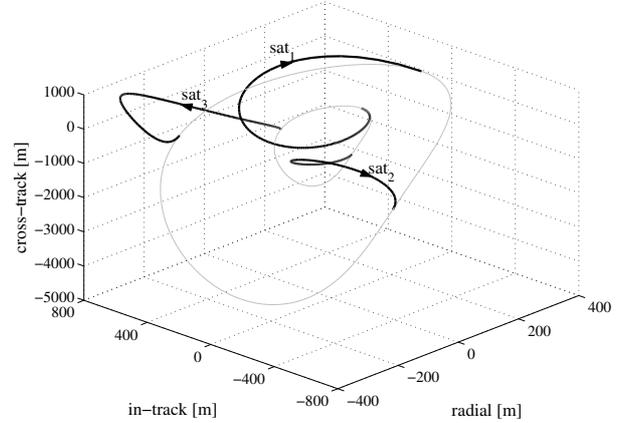
Fig. 4. Three satellites reconfiguration maneuver, Molnya reference orbit
