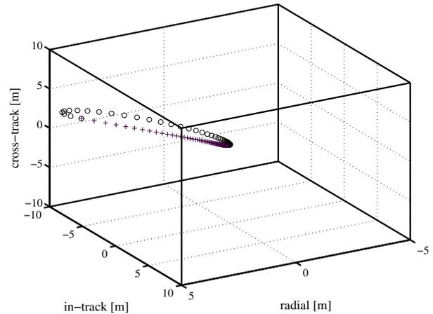
Fig. 6. Station keeping maneuver, Molnya reference orbit
