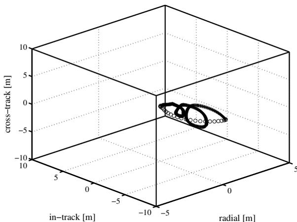
Fig. 5. Station keeping maneuver, circular reference orbit
