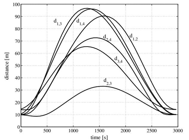
Fig. 2. Satellites relative distances during the maneuver
