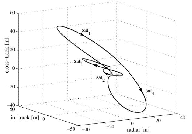
Fig. 1. Safe reconfiguration maneuver of four satellites
