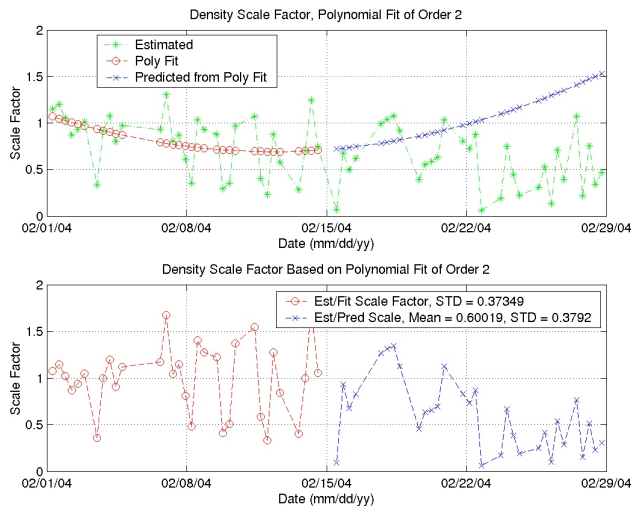
Fig. 12. Test density scale factor prediction from second order polynomial fit to first 14 days of arc.
