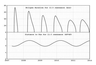
Figure 5: Eclipse duration vs. distance to Sun for 11:3 resonance
