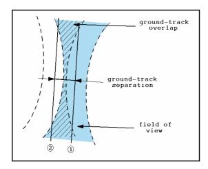
Figure 7: Ground-track overlap and separation concept.
