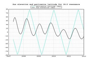
Figure 4: Sun elevation at pericentre for 18:5 resonance.
