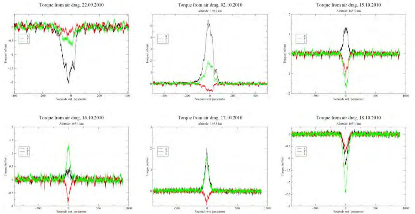
**Figure 8: Estimated Aerodynamic Torque during Different Experiments, from [3].**
