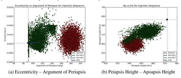
Figure 4: Distribution of (a) Mean Argument of Periapsis and Eccentricity and (b) Distribution of Apses Heights for Monte Carlo Simulation (5000 Sample Cases Shown).
