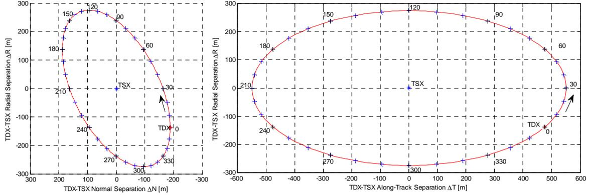
**Figure 2. TDX-TSX relative motion in the Hill orbital frame: Radial-Normal separation (left) and Radial-Along-track separation (right). The formation geometry ( $a \cdot \Delta e = 275\text{m}$ ,  $a \cdot \Delta i = 188\text{m}$ ,  $\varphi = 300\text{deg}$ ) was realized in the period from Jan. 12 to Mar. 29, 2012. The labels indicate the argument of latitude of the absolute orbit.**
