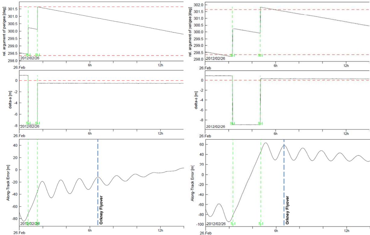
**Figure 8. Nominal ground-autonomous (left) and realized manual (right) in-plane formation control for the Pentland Firth acquisition on Feb. 26, 2012.**
