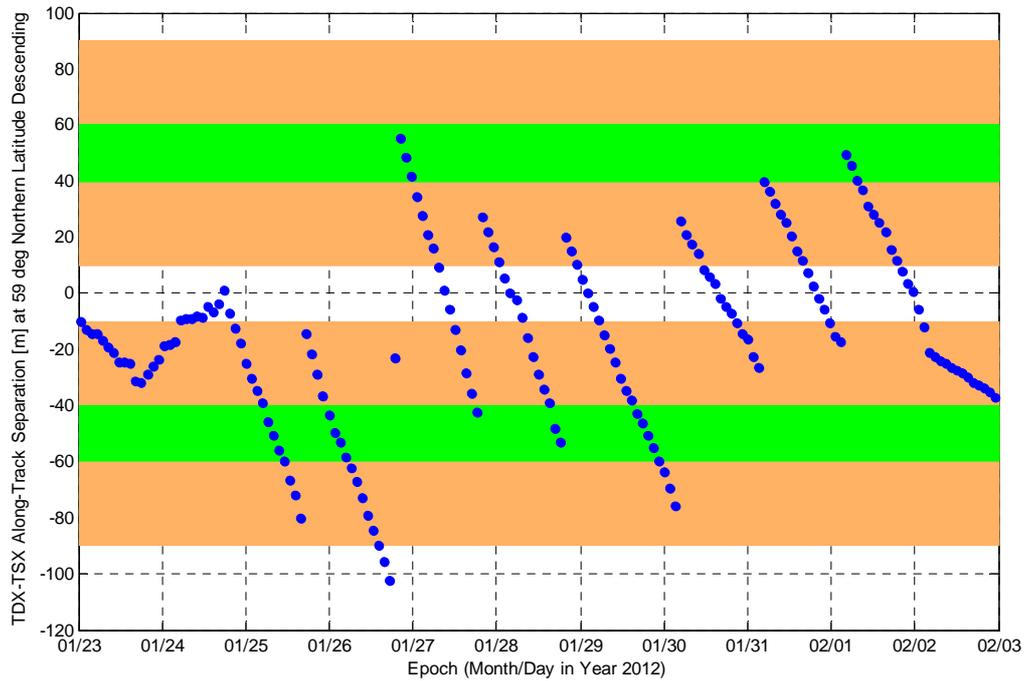
**Figure 7. Achieved TDX-TSX along-track separations at 59.5 deg northern latitude in 167 descending orbits during the cycle from Jan. 23 to Feb. 3, 2012.**
