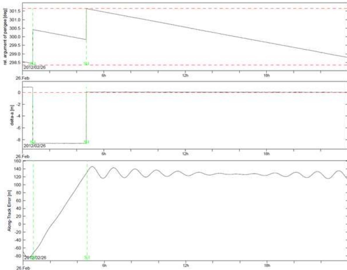
**Figure 11. Simulated formation change to acquire a +130m mean along-track separation.**
