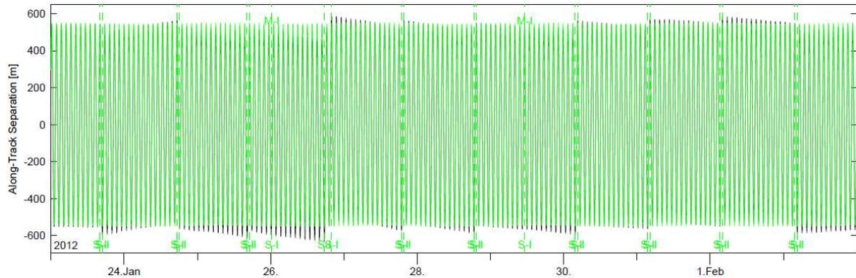
**Figure 4. Nominal (green) and real (black) TDX-TSX Along-Track Separation in the period Jan. 23 – Feb. 3, 2012.**
