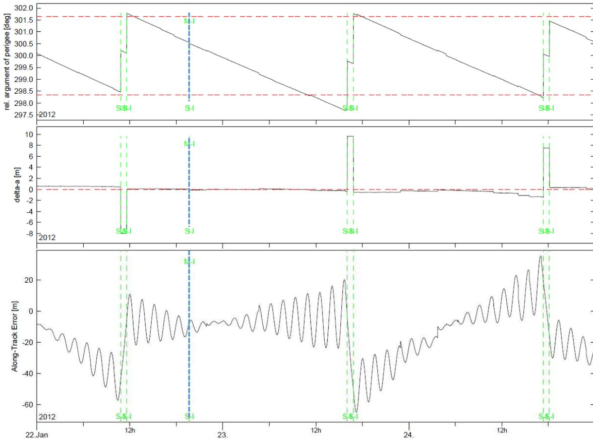
**Figure 3. TDX-TSX in-plane relative motion observed during the period Jan. 22-25, 2012. From top to bottom: relative argument of perigee, relative semi-major axis, and relative along-track error. The dashed verticals indicate common TSX/TDX maneuvers (blue) and TDX formation keeping maneuvers (green).**
