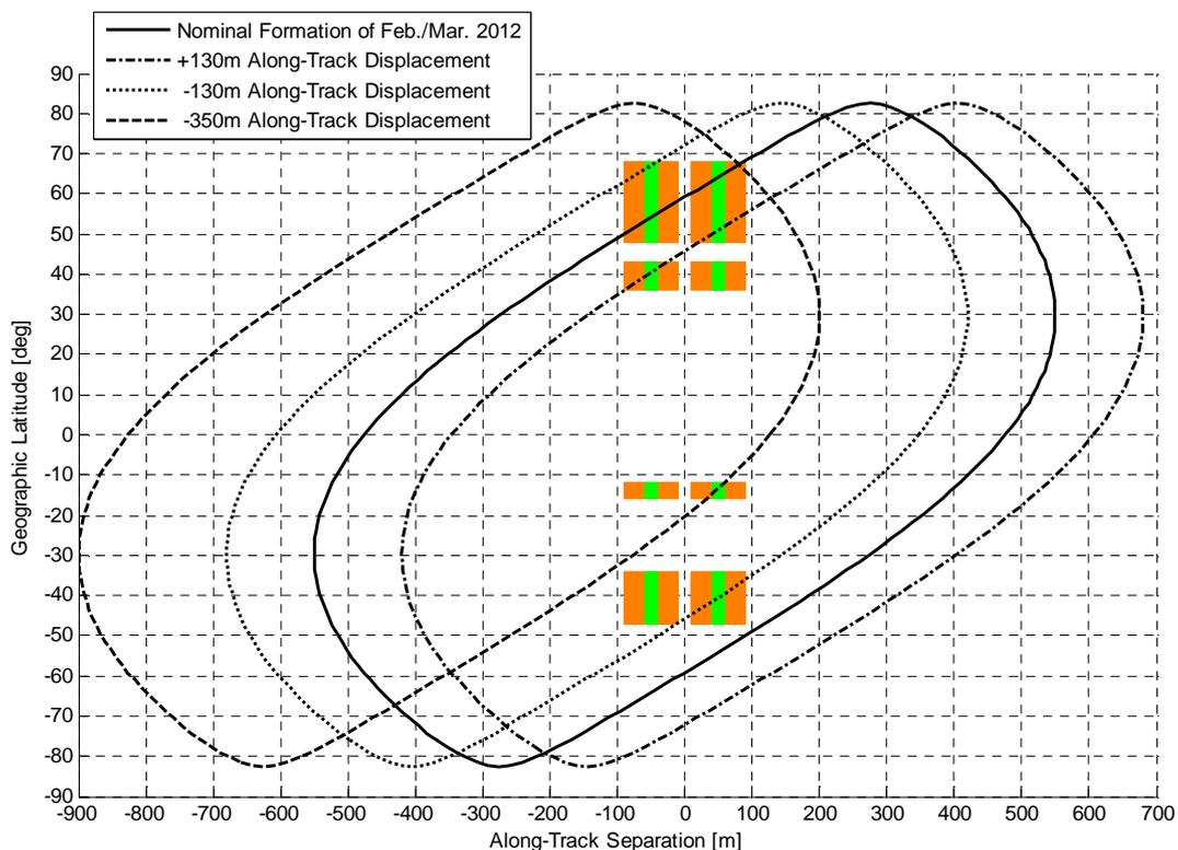
**Figure 10. Possible adjustments of the formation geometry from Feb./Mar. 2012 (persistent line) by means of pure along-track displacement. The rectangles illustrate oceanographic ATI site groups with optimal (green) and tolerable (orange) range in along-track separation. The northern energy sites are acquired in descending orbits while the southern sites are observed in ascending orbits.**
