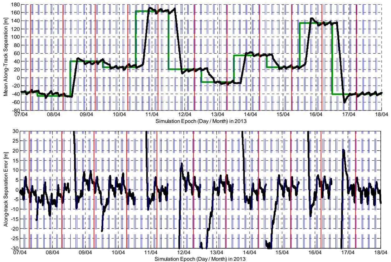
**Figure 12. TAFF control performance in ATI mode: 11 day simulation with several reconfigurations of the relative mean along-track separation: Top: target (green) and simulated (black) mean along-track separation. Bottom: Achieved control accuracy. The TAFF maneuvers are depicted as dashed blue lines. The ATI acquisition epochs are marked as red lines.**
