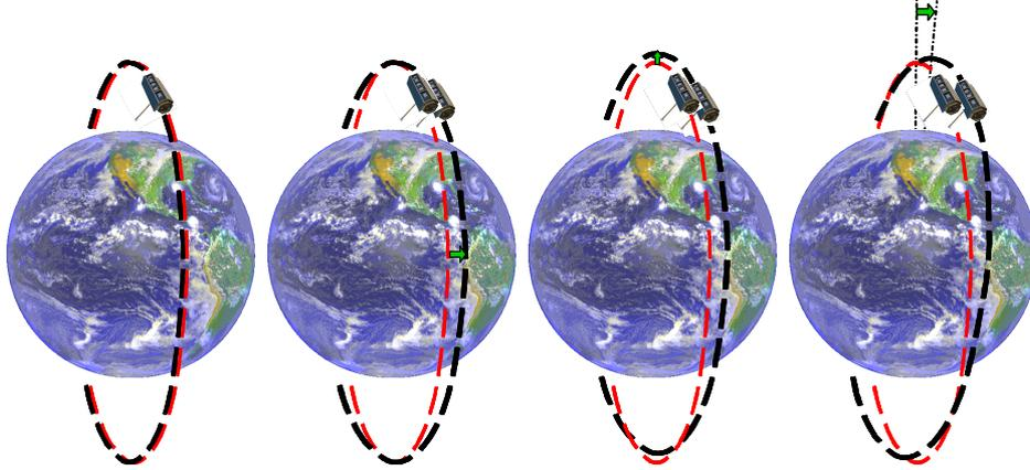
**Figure 1. Formation building with relative eccentricity / inclination vector separation. From left to right: (1) identical orbits, (2) maximum horizontal separation at equator crossings by a small offset in the ascending node (green arrow), (3) a small eccentricity offset causes different heights of perigee / apogee and hence yields a maximum radial separation at the poles. (4) Optional rotation of the argument of perigee to achieve larger baselines at high latitude regions.**
