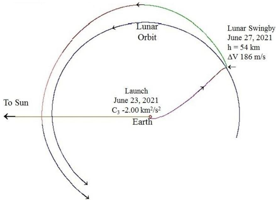
**Figure 10. The trajectory shown in Fig. 9 in a rotating ecliptic plane view with a fixed horizontal Sun-Earth line.**
