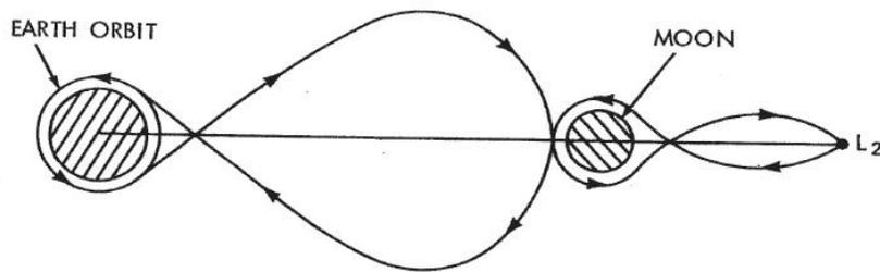
**Figure 3. Mission Profile for a Lunar Shuttle System with (Earth-Moon L2) Halo Orbit Staging. From [8] and Fig. 3-3 of [10].**
