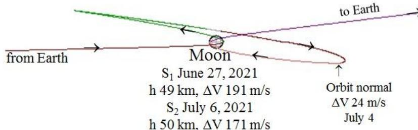
**Figure 6. View from the Earth of the trajectory shown in Fig. 4 and 5. The horizontal direction passing through the Moon is the lunar orbit plane, while the vertical direction is perpendicular to the lunar orbit plane.**
