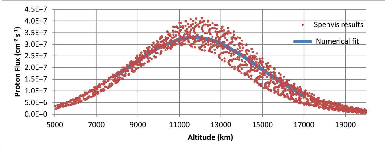
**Figure 5: Fit of the 1 MeV proton flux predicted by SPENVIS [6] for a GTO to GEO transfer.**
