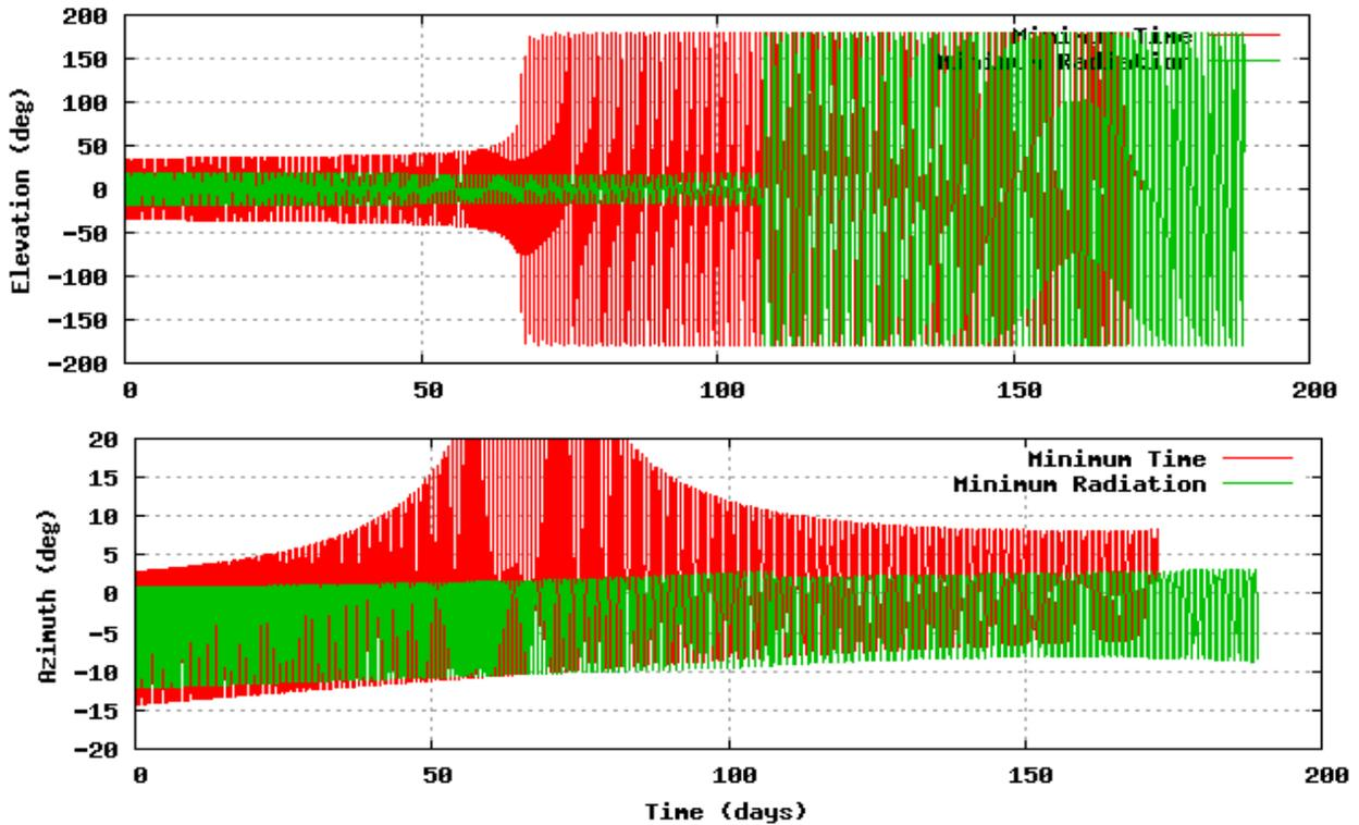
Figure 7: Time history of elevation (= in-plane component, top panel) and azimuth (=out-of-plane component, bottom panel) of the thrust vector during a minimum time transfer and for a minimum radiation transfer from GTO to GEO.
