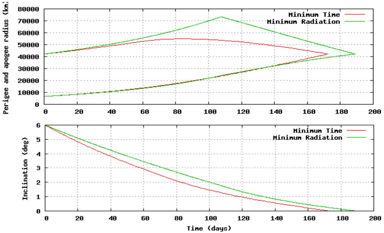
Figure 6: Inclination, perigee and apogee altitude evolution for a minimum time and for a minimum radiation transfer from GTO to GEO.
