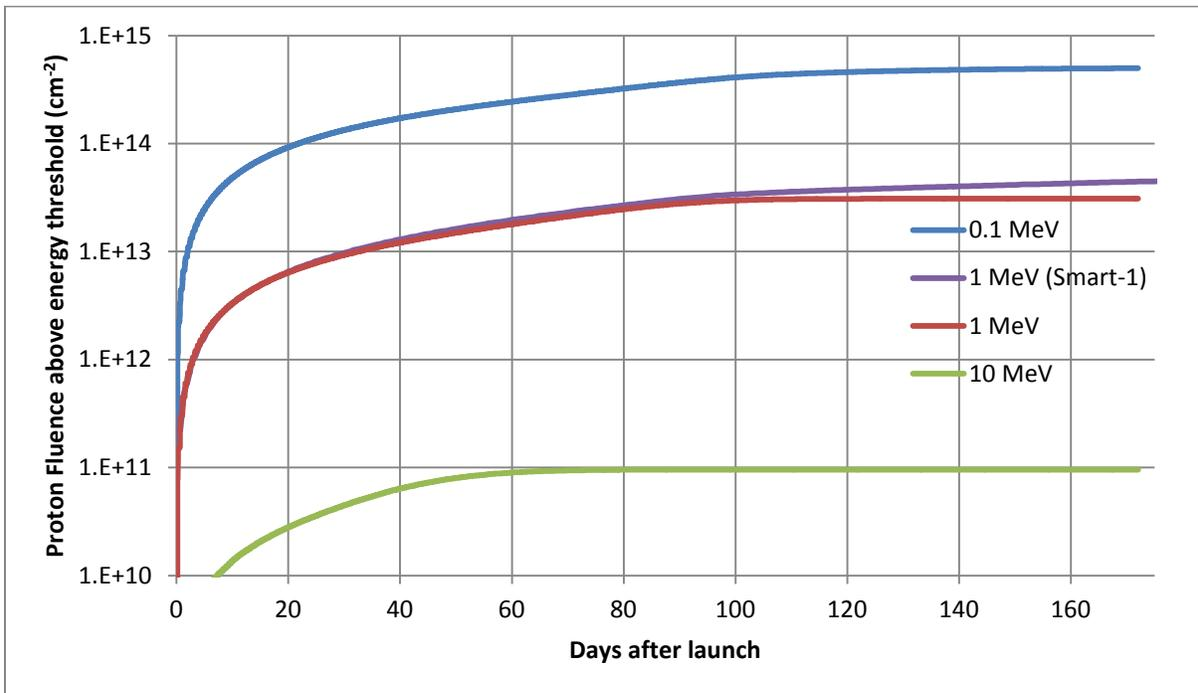
**Figure 4: Proton fluence during a SEP transfer from GTO to GEO (including simulated fluences for the Smart-1 trajectory)**
