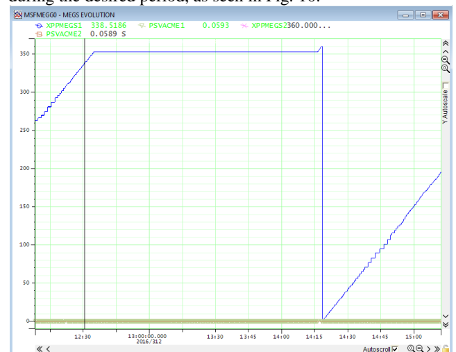
Fig. 10. Solar panel rotation around the revolution in inertial attitude.
